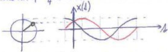
Complex amplitude (initial point position for  $t=0$ ) will rotate by  $+\frac{\pi}{4}$ . Furthermore, vertical axis in right part of the picture will move by  $\frac{\pi/4}{2\pi} \cdot T = \frac{T}{8}$  to the right.
