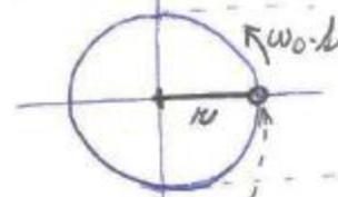
point rotates with  $\frac{\omega_0}{2\pi}$  revolutions/sec, the position of the point can be seen in complex plane and expressed as  $a(t) = r \cdot e^{j(\omega_0 t + \phi)}$
