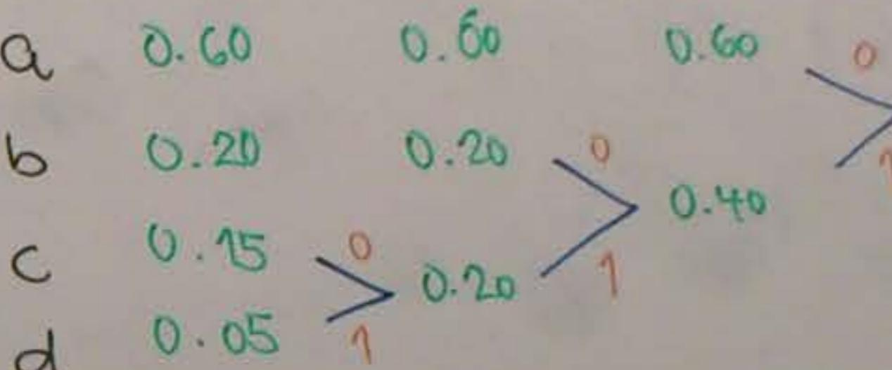
$$\begin{aligned} a &\rightarrow 0 \\ b &\rightarrow 10 \\ c &\rightarrow 110 \\ d &\rightarrow 111 \end{aligned}$$
